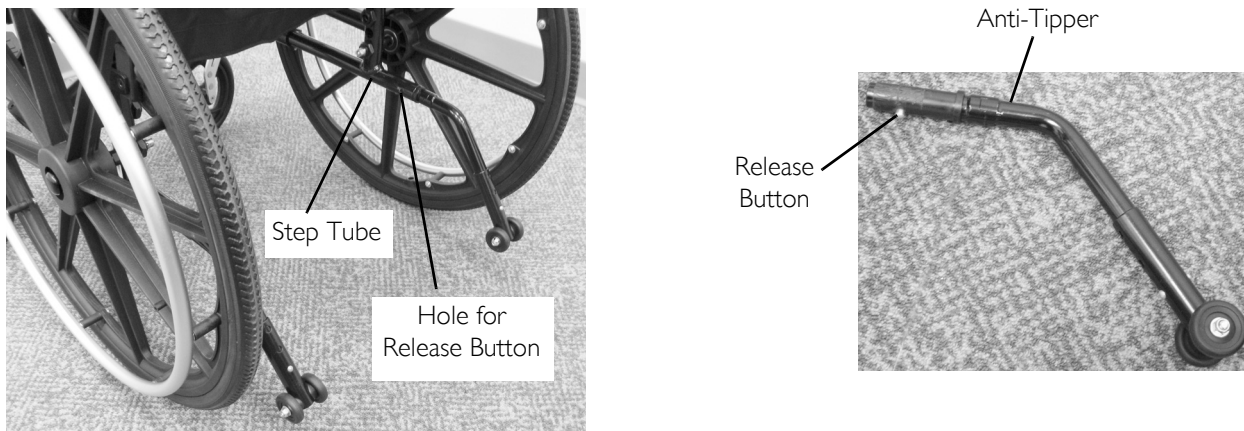
FIGURE 10.1 Installing Anti-Tippers
